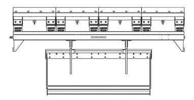
4. Once the D-Rings have been welded to the inside of the bucket use a Chain and Chain Binder to secure the plow to the Bucket. Two Chain Binders can be used on the bucket depending on the depth of the bucket as shown below.
